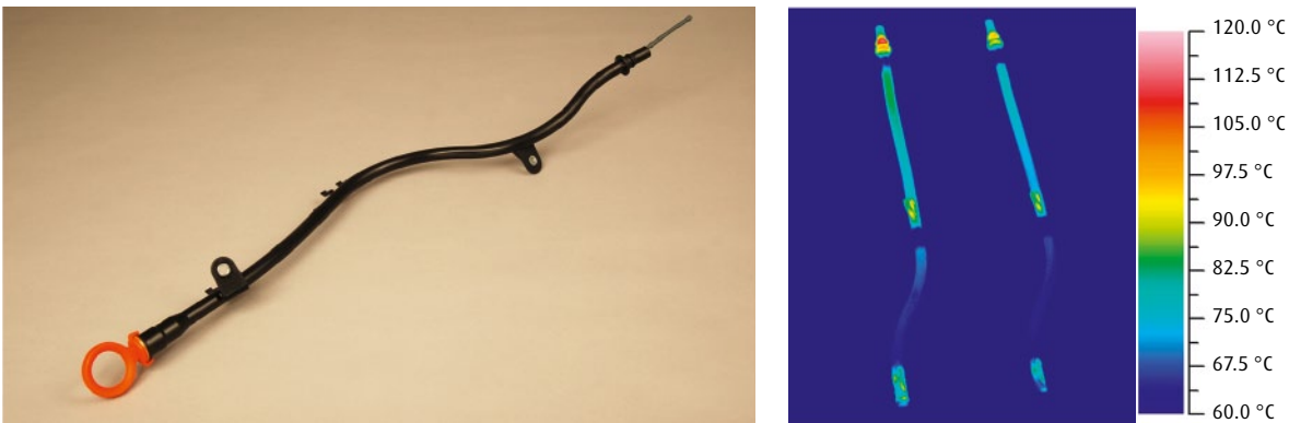
Fig. 5. At the end of the cycle, the temperature of an injection-moulded dipstick guide tube made from PA6.6 GF30 CO_2 is much lower than the normal demoulding temperature for such materials, as shown here by the thermal image captured immediately in the 2-cavity mould after the moulding process.
