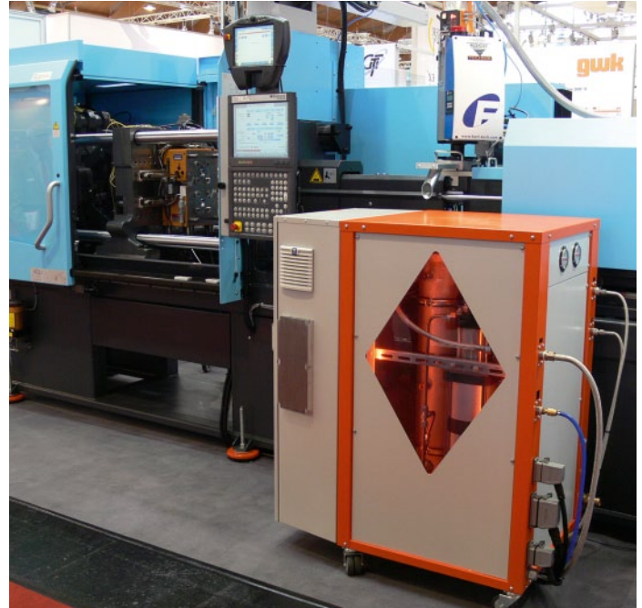
Fig. 7. The installation for dynamic mould temperature control combines rapidly alternating heating and cooling cycles at temperature gradients of up to 20 K/s.
