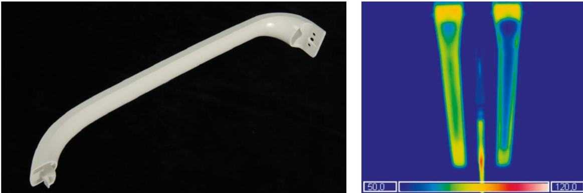
Fig. 4. The cycle time for this refrigerator handle was shortened by more than a third. This thermal image, captured immediately after the moulding process, shows the higher temperature of an injection-moulded handle produced with N_2 (left) compared with that achieved with CO_2 (right).
