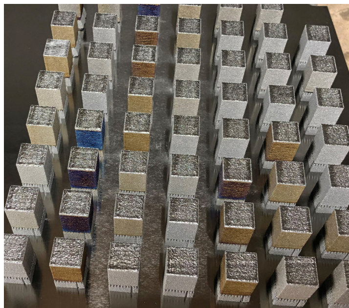
Nitinol cubes showing discoloration caused by oxidation from too high or inconsistent O 2 levels in the printing chamber.
