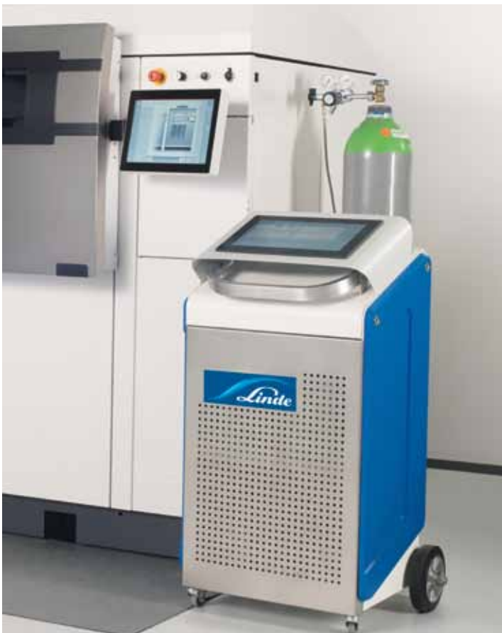
The ADDvance® O 2 precision ensures the atmosphere inside the print chamber.
